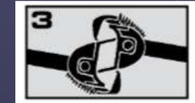
4. Pull forward, leaving the car(s) where desired. Couplers will automatically return to normal coupling position.
