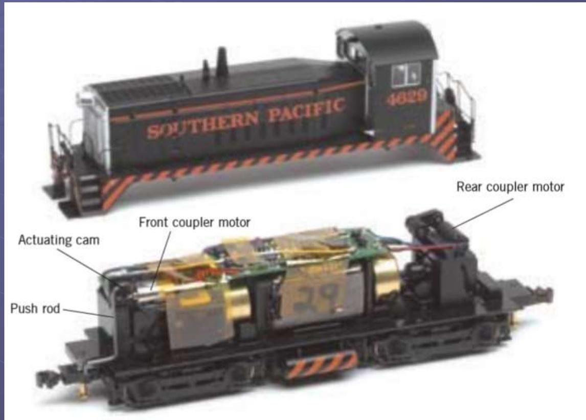
Retro-fit Digital Command Control operated uncoupling kit for Life-Like Proto 2000 SW-style locomotives.
